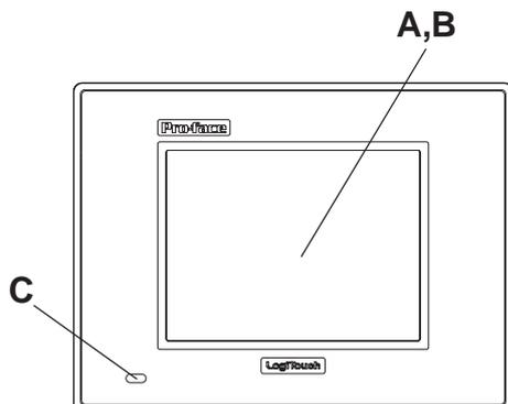
A : Display : Displays controller and user-created screen data.
